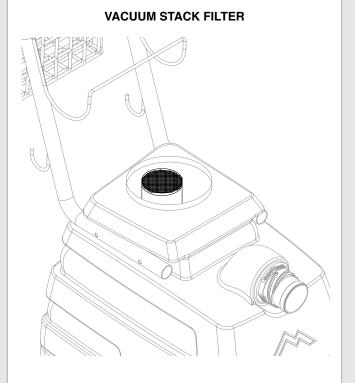
The Mytee-Lite's™ internal filter must be cleaned regularly and is located in the recovery tank. Twist the filter to remove then clean and replace. If the filter is torn or damaged, replace with a new one.
