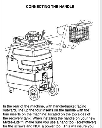
do not strip the hole and puncture the recovery tank.
