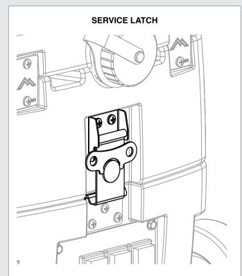
To open lower housing flip-up latch that is located in the back of the unit. Twist counter clockwise for release. To close unit, place latch, twist clockwise and press latch to secure.
