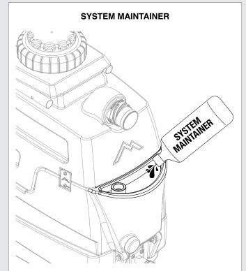
Weekly flushing of the solution system with Mytee System Maintainer helps keep lines clean and prevents chemical build-up, improving pump life, performance and pressure.
